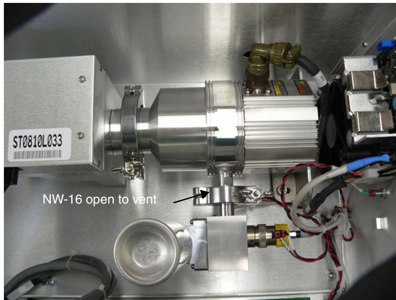
Figure B-76 NW-16 Vent
