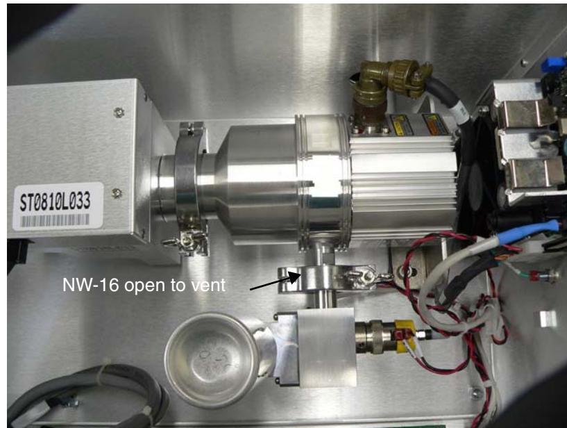
Figure B-48 NW-16 Vent
