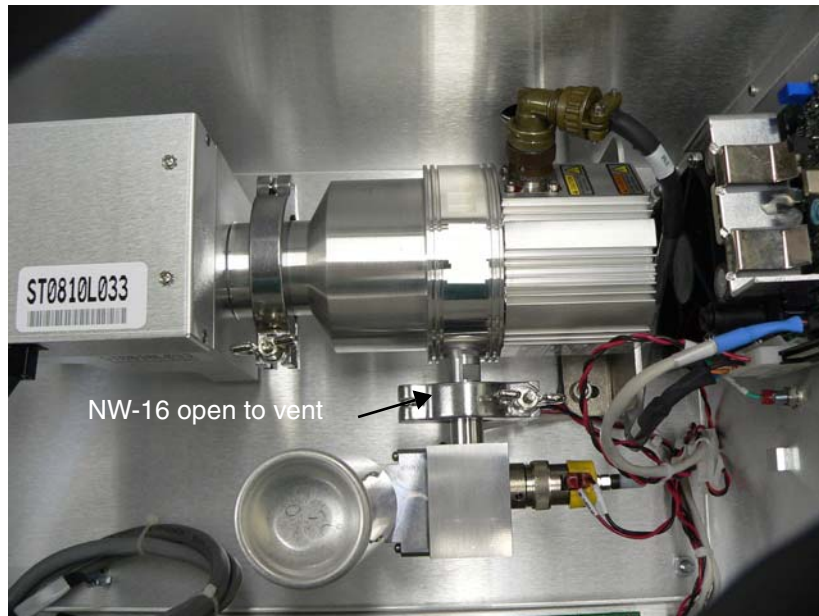
Figure B-59 NW-16 Vent
