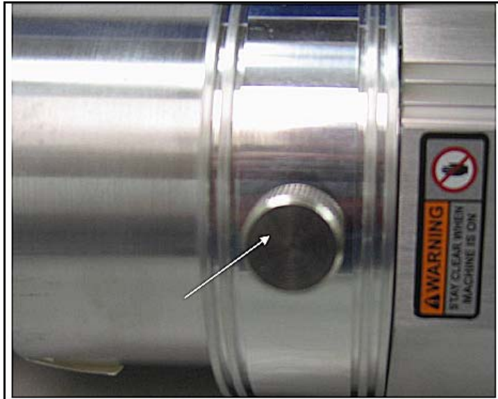
Figure B-2 NW25 Clamp with Calibrated Leak Not Present
